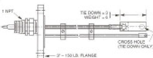
**L116** Flange Mounted Dual Flexible Probe Availability: TW, KW
